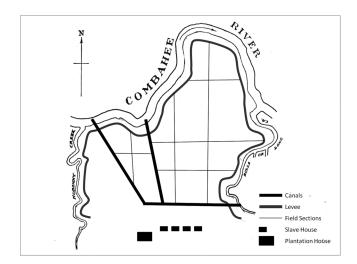
Figure 4. Hypothetical map constructed by a student. Careful step-by-step consideration for field development would include locating levees, canals, floodgates, field sections, and housing.
